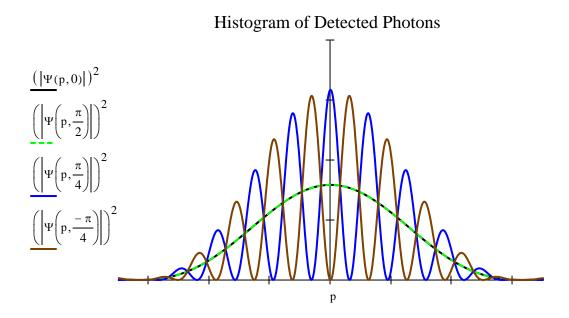
Regarding the last demonstration, the reason for the restoration of the interference fringes is that the "which-way" information provided by the crossed polarizers has been lost or erased. The vertically and horizontally polarized photons from slits 1 and 2 both have a 50% chance of passing the diagonally or anti-diagonally oriented third polarizer. Thus, knowledge of the origin of a photon emerging from the third polarizer has been destroyed.
